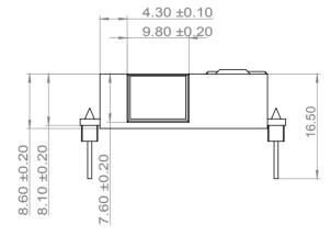
Pin is the common standard type with square cross section.
