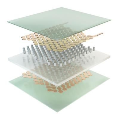
Figure 1: Picture showing the layers (Package, Contacts, Thermopiles, Substrate, Interconnects) of gSKIN® Heat Flux Sensor (thermopiles are highly integrated in the sensor substrate, which leads to high sensitivity sensor modules).
