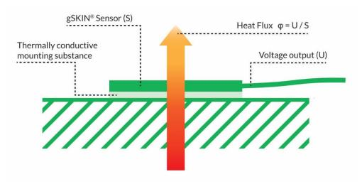
Figure 2: Schematic diagram of mounting and functionality of a gSKIN® Heat Flux Sensor.
