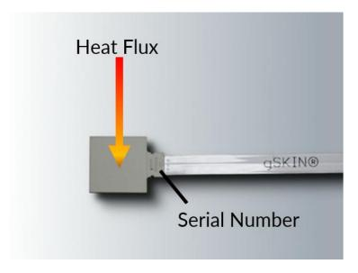
Figure 3: This placement shows the positive side of the sensor (i.e. assuming a heat flux from top (hot side) to bottom (cold side), this sensor will generate a positive voltage signal). Alternatively, the correct sensor orientation can be determined by placing the flex print in such a way, that the serial number is not visible.
