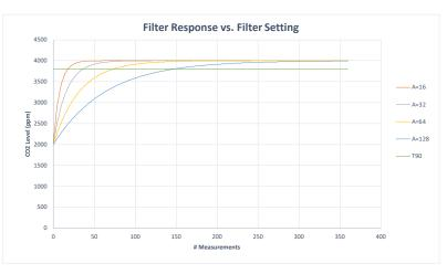
The graph above shows the effect of the filter on response times. Increasing the filter setting increases the measurement output response time.  $T_{90}$  is the time to 90% of reading. The SprintIR<sup>®</sup>-6S takes 20 readings per second. The flow rate was set at 0.2l/min.
