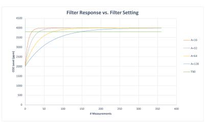
The graph above shows the effect of the filter on response times. Increasing the filter setting increases the measurement output response time.  $T_{90}$  is the time to 90% of reading. The ExplorIR<sup>®</sup>-M takes 2 readings per second.
