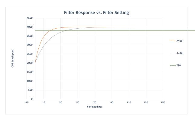
The graph above shows the effect of the filter on response times. Increasing the filter setting increases the measurement output response time.  $T_{90}$  is the time to 90% of reading. The CozIR®-LP2 takes 2 readings per second. The CozIR®-LP2 sensor will also output the raw unfiltered  $CO_2$  measurement data. This data can be post processed using alternative filter algorithms.
